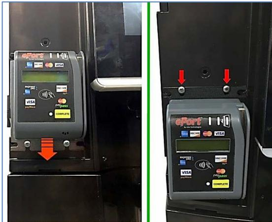
5. Install the appropriate cover (for card reader being used) onto the front of the door, and secure it in place with a screw from the inside of the door (at top center of card reader opening).
