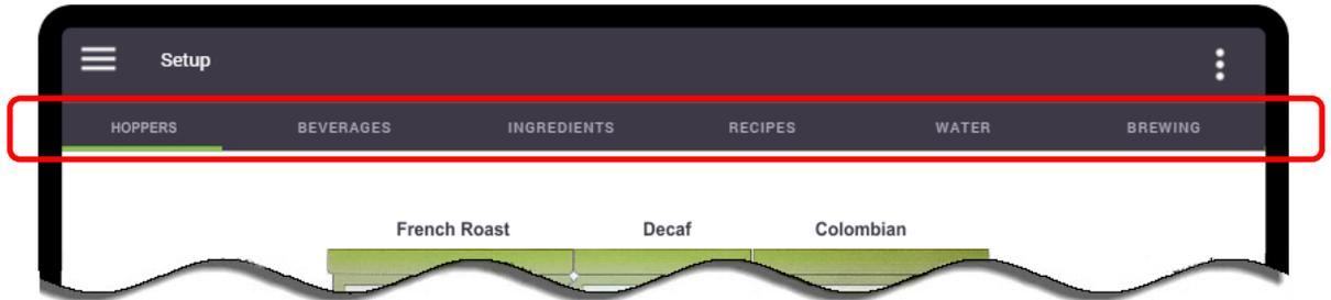
If multiple tabs are available, the currently active tab is identified by a green line directly beneath the sub-menu name, which also appears white instead of gray.
