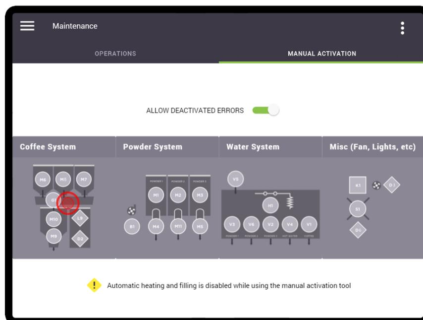
A new screen now appears showing all of the components that are part of the Coffee System. Each component is identified by a unique component code.
