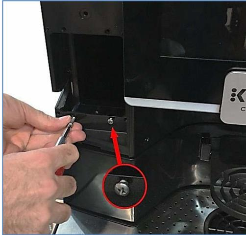
4. Pass the card reader wiring to the rear of the door (through the card reader opening), and then slide the bottom of the card reader onto the two partially inserted screws. Once done, secure the top of the card reader with two screws, and then tighten the two lower screws to secure the bottom of the card reader.
