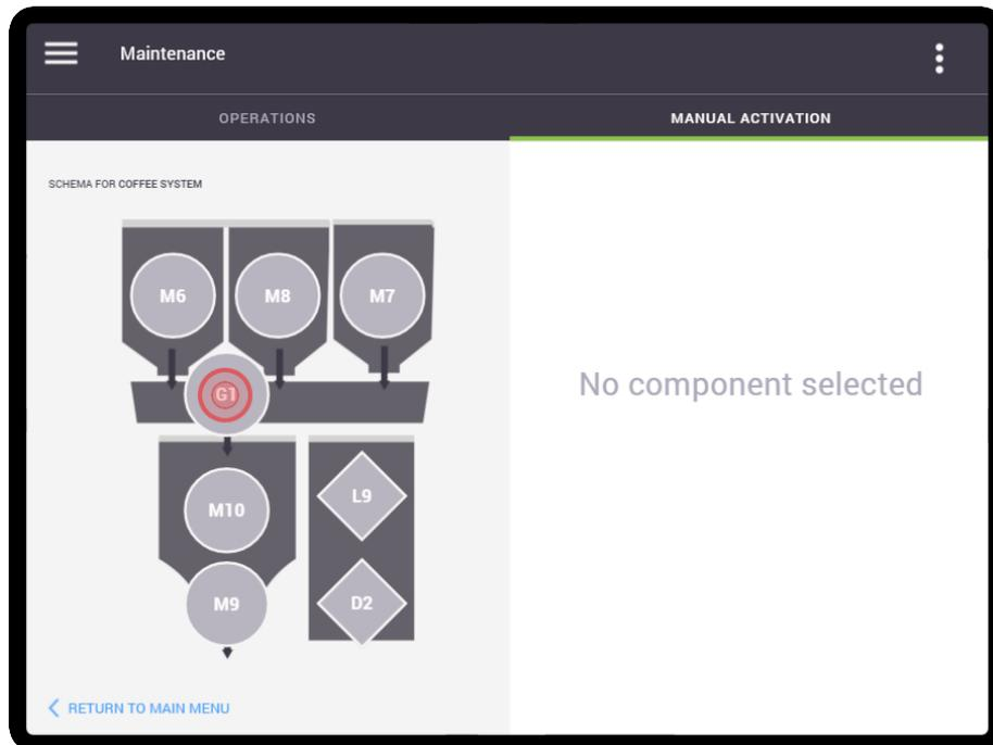
The testing options now appear on the right section of the screen. In this example, the only option available is to activate the grinder for 3 seconds.
