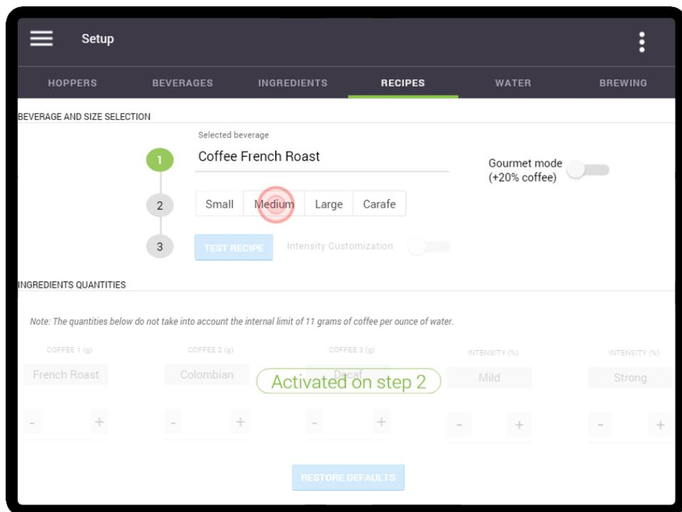
Notice that the French Roast setting is now active (not grayed out) in the 'Ingredients Quantities' section of the screen. This indicates that this setting can now be adjusted. Also note the 'Intensity Customization' setting on Line 3. This is used to adjust the 'Mild' and 'Strong' strength coffee settings. Tap on the slider to activate it.
