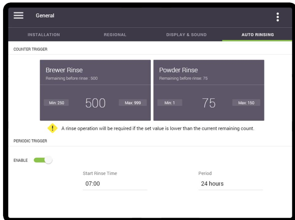
To change the frequency, tap on the desired option and input the new setting. Once you are finished, tap the 'Done' button to save your new setting.
