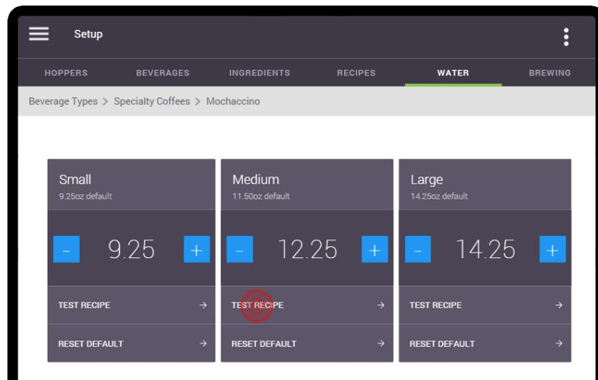
5. To reset a specific setting back to its default, press the **'Reset Default'** setting for the corresponding cup size. *The original default setting is shown beneath each cup size.*
