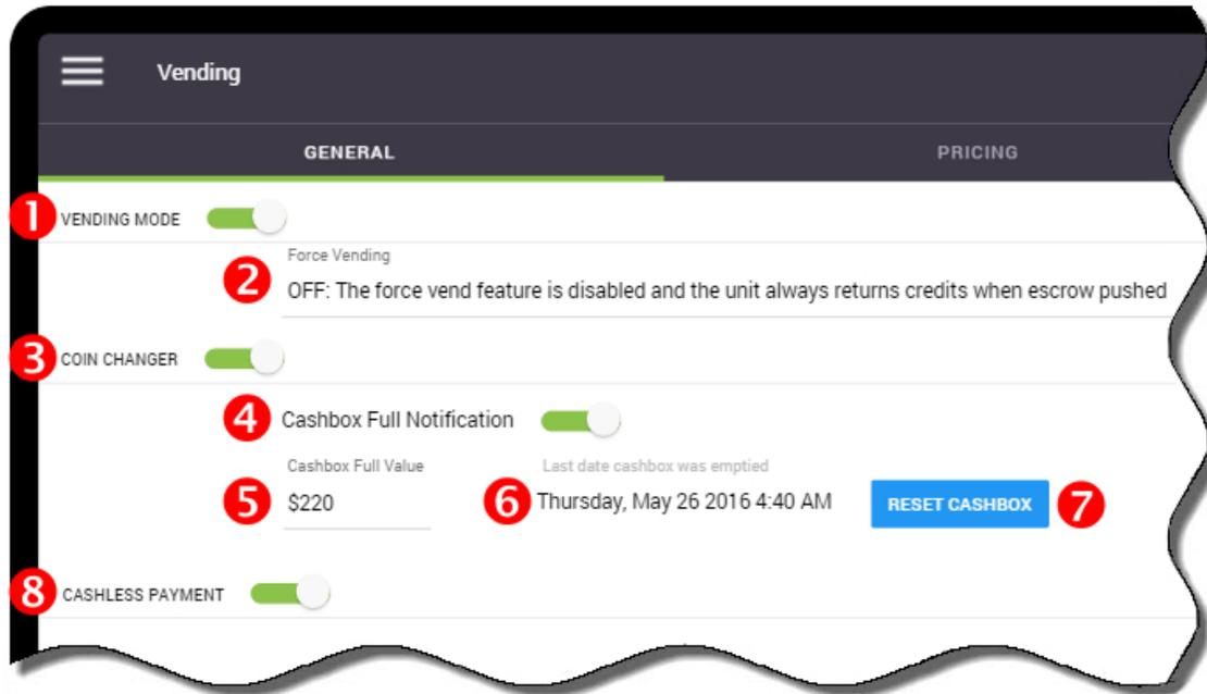
The **Vending Mode** slider **1** enables or disables the vending functions - vending is enabled when the slider is green.
