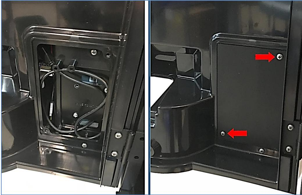
12. Bundle and stow any excess wiring inside the opening at the top of the door, and reinstall the cover using four screws.
