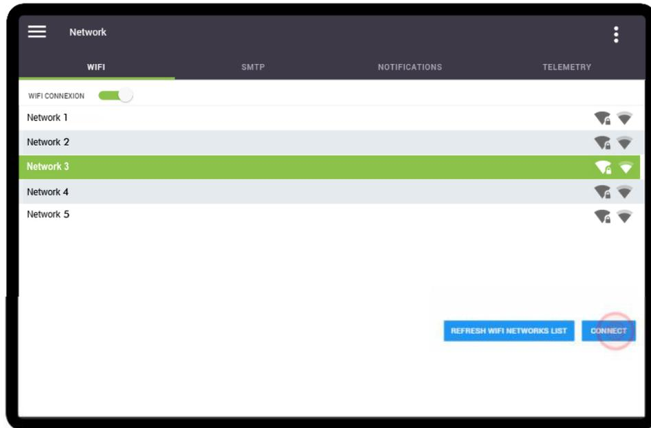
4. The keyboard appears and you must now type in the required password to connect to the selected network. Once done, tap the 'Accept Change' button.
