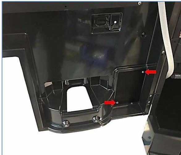
2. Remove the screw at the top center of the opening, and then remove the original full cover from the outside of the door.
