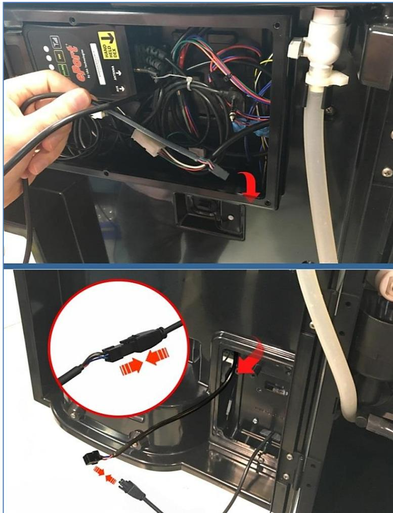
11. Bundle and stow any excess wiring inside the opening for the card reader (at the bottom of the door) and reinstall the cover using two screws.
