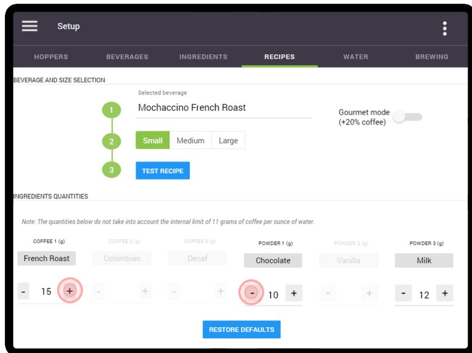
7. To brew a test beverage using the new settings, place a cup on the cup stand and tap on the blue 'Test Recipe' button on line 3. The Momentum will now dispense a Mochaccino French Roast that you or your customer can taste test. If further adjustments are required, make the changes and the test the beverage again until you get the required results.
