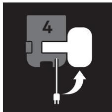
Rotate the base to desired position, slide the base into the brewer to lock in position. Reposition power cord into slot.
