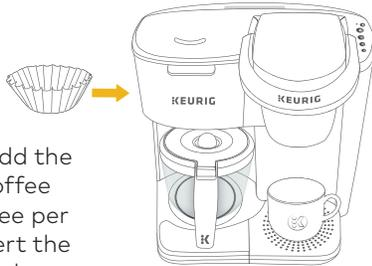
**NOTE:** The maximum capacity for regular ground coffee is 15 tablespoons and 12 tablespoons for decaf. Exceeding this amount may cause overflow.
