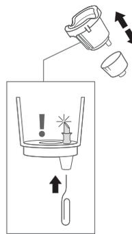
Remove the pod holder assembly and detach the funnel. Locate the exit needle on the inside bottom of the K-Cup® pod holder. Insert a straightened paper clip into the exit needle to loosen any coffee grounds.
