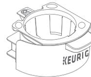
Remove the filter basket drawer from the brewer. Remove and discard the paper filter and ground coffee. The filter basket and filter basket drawer should be washed in warm, soapy water and rinsed thoroughly. Dry all parts after use.
